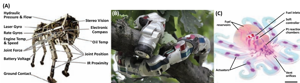
Fig. (1). Traditional rigid robots, Soft-imitation robots and Soft robots. (a). BigDog [1]. (b). Snake-like robot [6]. (c). Octobot [9].
