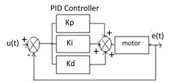
Fig. (1). Block diagram for PID controller.
