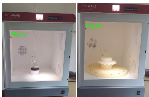
Fig. (1). The MWI devices (a) the monomode reactor MW (b) the multimode reactor MW.
