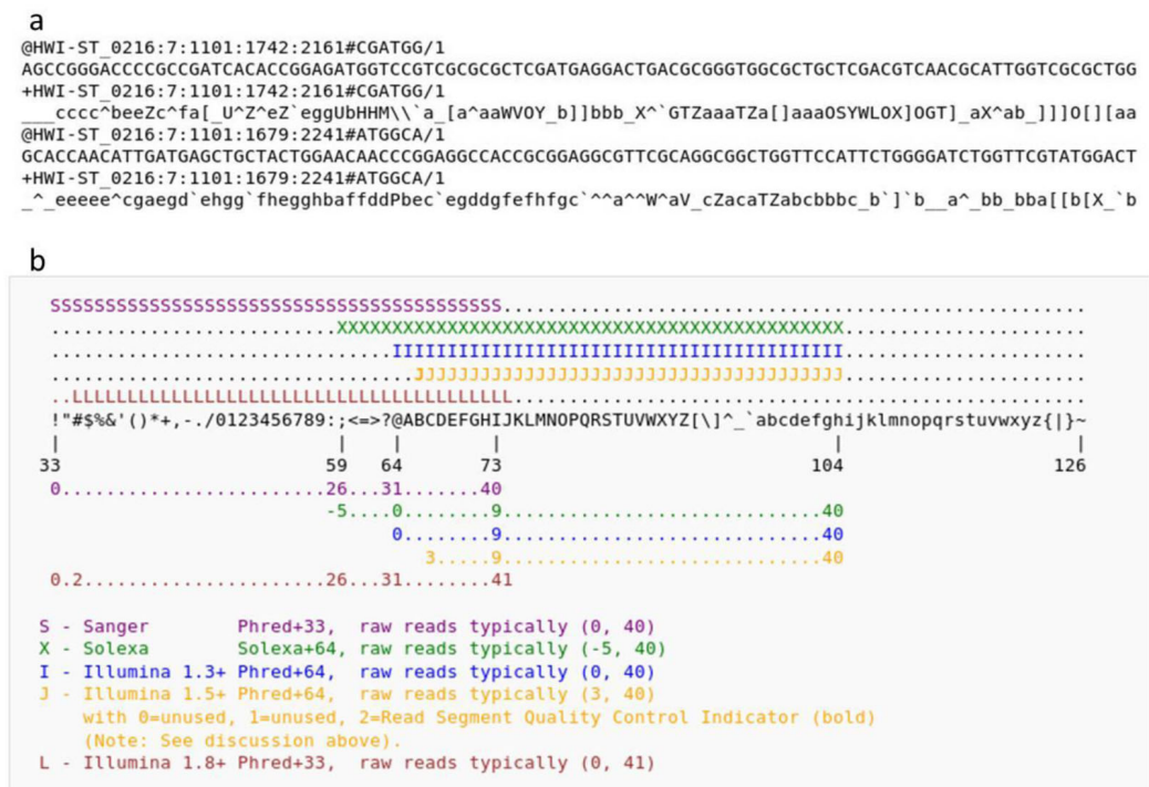
Fig. (2). An example of Fastq format (a). Each sequence is represented in four lines, sequence header, sequence, quality header, and quality line. Various schemes can be used to encode quality scores (b). The numeric scores are converted to the corresponding ASCII code.
